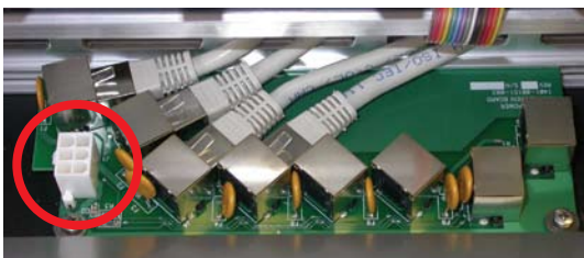
Figure 1-5: Element connection panel. Circled connector is for power/data cable; RJ-45’s connect to fader and accessory modules.
