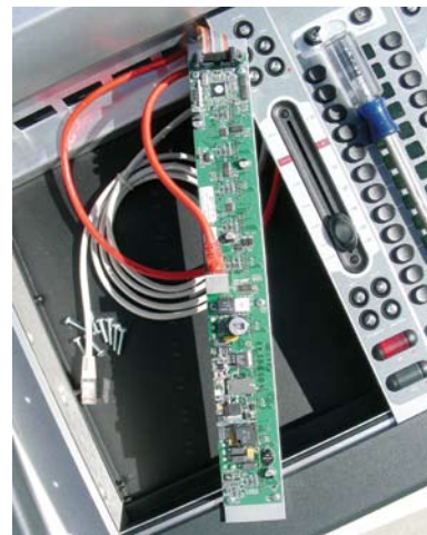
Figure C-11: Reverse view of connected module. Note ribbon cable is connected “tail-up”.
