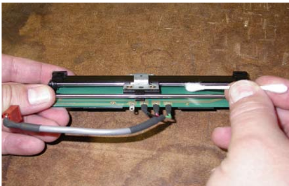
Figure C-19: Cleaning the fader glide rails
