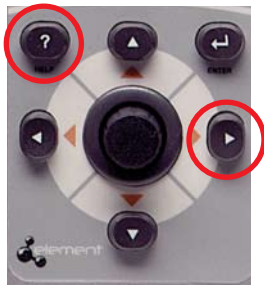
Figure C-13: Press and hold these keys for 5 seconds to enter module diagnostic mode.
