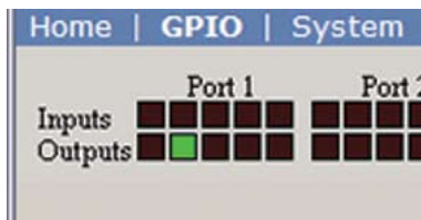
Figure 2-6: GPIO status indicators
