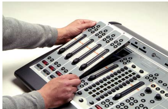
Figure C-16: Tilt module up to remove from frame.
