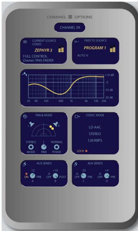
Figure 4-6: Channel Options screens. Information displayed differs based on the type of source currently assigned to the active fader. Shown clockwise from top left: Line Source Channel Options screen, Mic Source Channel Options screen, Phone Source Channel Options screen, Codec Source Channel Options screen.
