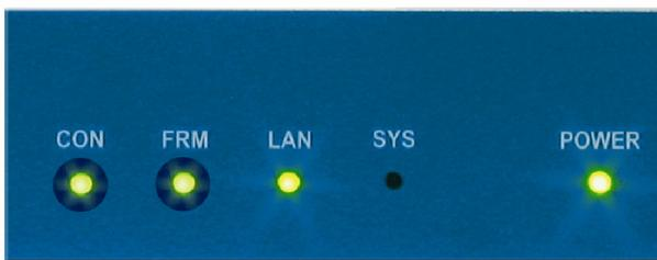
**CON led:** When this led is on, It indicates that the unit is connected.
