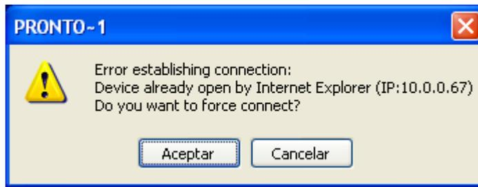
It is possible to get the control by pressing OK. Then, the connection of the old owner will be closed and the unit will be blocked for new controller.
