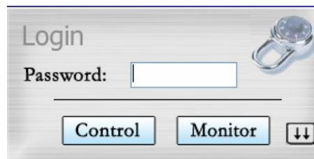
If a unit is already being controlled by a web page and we try to get the control from another web browser, a message will appear. This message will indicate that the unit is already being controlled from another PC and the IP address of this computer.
