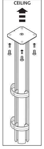
Turn the MSS Pole to mount the ceiling adapter plate using the M10 countersunk screw. The plate comes with holes in the corners for mounting it at the ceiling with another four countersunk screws. Cable clamps are included in the scope of delivery.
