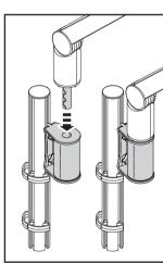
You can mount up to four Mic Arm to MSS Pole Adapters (#YT3213) and respectively microphone arms on a single MSS Pole due to its four profile slots. The resulting 'tree' will be a perfect support for a guest table. Mount one MSS Pole in the centre and let it hold up to four microphone arms by using these adapters.
