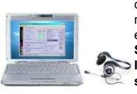
The reporter, correspondent or remote (OB) engineer uses the STL-IP Connect IP Codec software on a standard Laptop or PC
